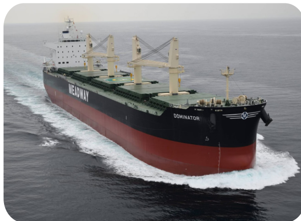
Supramax bulk carrier "Dominator", 63.652dwt, built 20241, Imabari Shipyard
